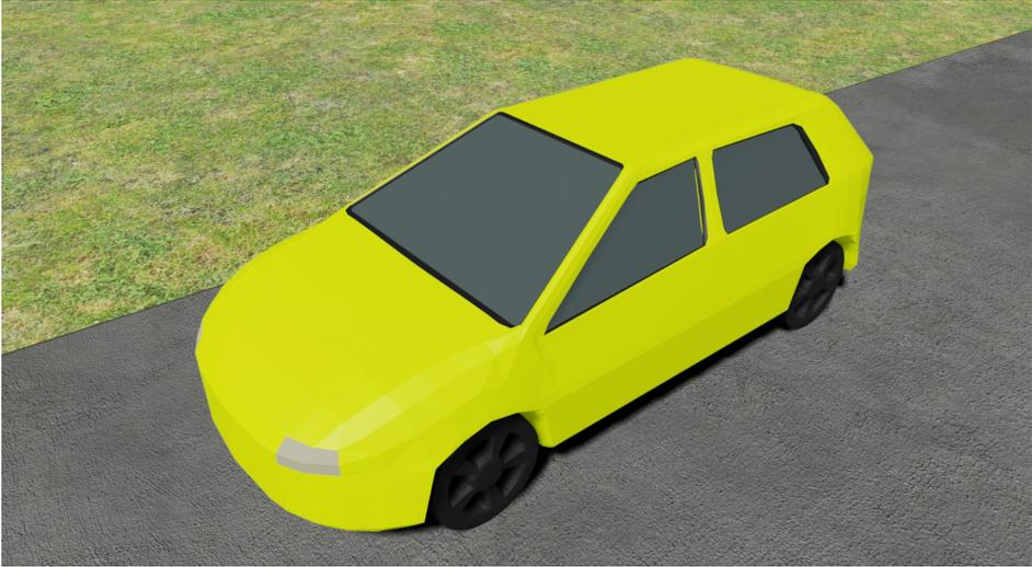
**Figure 3.4:** *An image illustrating one of our yellow Volkswagen Golf vehicles. This vehicle is built upon the NVIDIA PhysX vehicle and has the same physical attributes, e.g., height, torque, width, as the sedan vehicles.*
